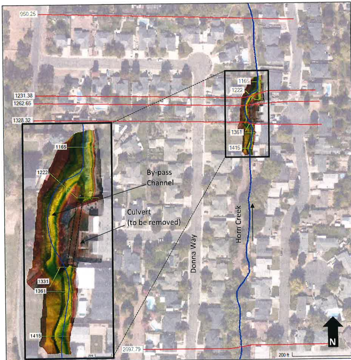
Figure 1. Vicinity map showing topography collected by Neathamer relative to effective (red) and revised (green) cross-section alignments.
